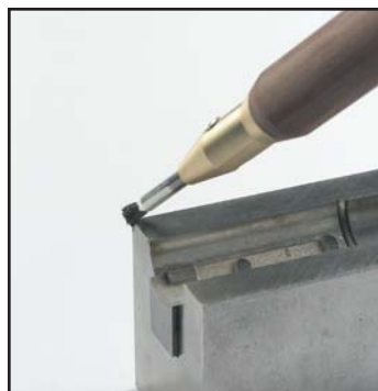
Three-point corner welding
